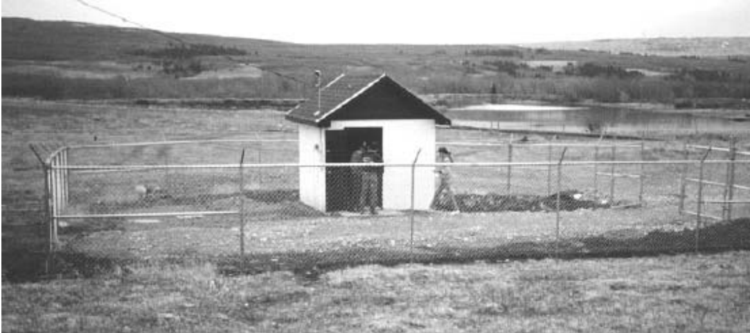
Figure 10.2.1 – Fencing Protection Around a Well
